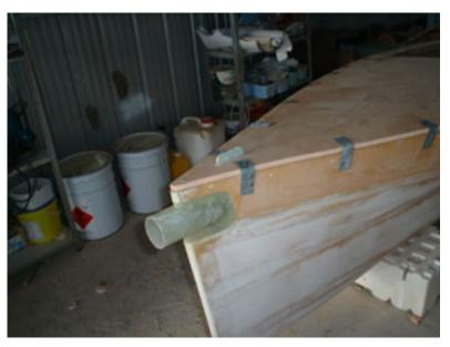
The aft deck and the side decks are attached. An edge is built using foam between the fore and aft decks.
