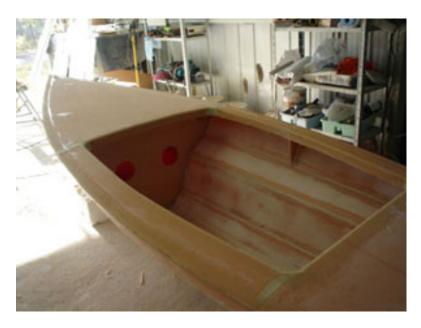
A mast support tube is made from glass laminated over a metal tube covered with cardboard or similar.
