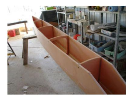
The sloping transom is added and taped to the hull.
