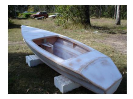
The inside of the hull was filled ready to paint.
