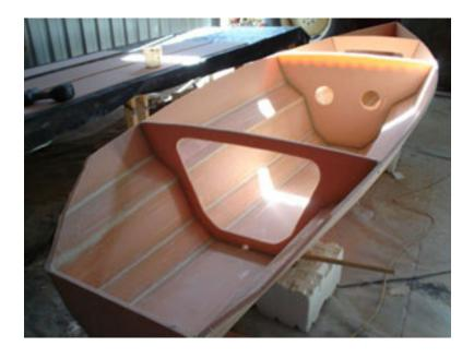
A plywood stinger to strengthen the deck was added between bulkhead no.2 and no.4.
