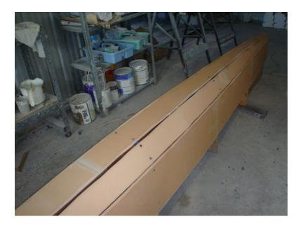
The panels added to the frame and joined with drywall screws (foam) or staples (plywood).
