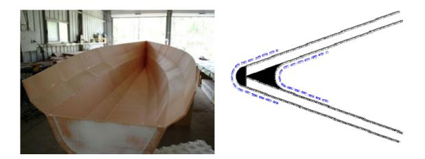
Because it is narrow and difficult to reach, it can be a problem finishing inside the stem. The best way we have discovered is to sand the inside of the bow and use a section of pre-wetted double bias glass laid in as shown below. When the glass hardens resin mixed with aerosil is poured into the gap. This should be done gradually as the resin will generate considerable heat with a possibility of catching fire.
