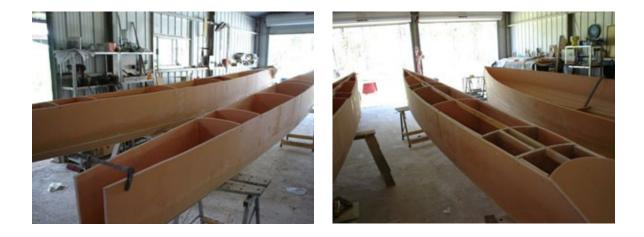
The laminated panels are too stiff to bend over the deck shape. We attached scraps of foam on the outside of the hull to temporarily hold the deck. The foam was joined to the right length and drywall screws were used to attach the deck foam to the hull. Care was taken to not screw into the hull itself. The deck was laminated with glass cloth and resin on the outside. When the glass hardens still attached to the scrap foam. The scraps were removed and the inside of the deck was laminated.
