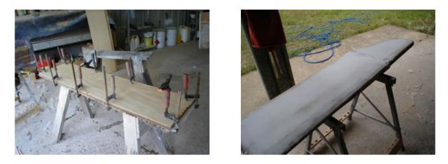
The centre board and the rudder are made using layers of plywood. Two pieces of 12mm plywood are laminated using a couple of layers of glass cloth and epoxy resin between. When the board is shaped the glass inside gives a sharp finish to the trailing edge directions in the plans.
