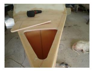
The anchor locker is cut and finished inside. A support to hold the fore stay is added to the forward bulkhead. The foam around the edges is removed, filled and the plywood-insert added hold the anchor lid.
