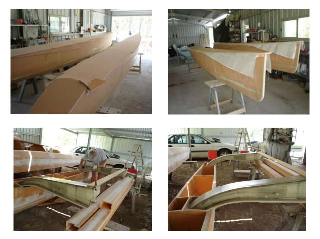
The floats are levelled and the beams are set up through the appropriate bulkheads.
