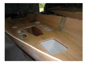
The cabin top is temporarily joined with metal strapping, tacked, filleted and taped. The hole for the hatch is cut out and hatch surround added with scraps of foam laminated strengthened with unidirectional glass.
