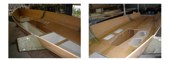
A temporary frame is set up for the cabin roof using the main cabin bulkhead, the forward bulkhead and scrap plywood.
