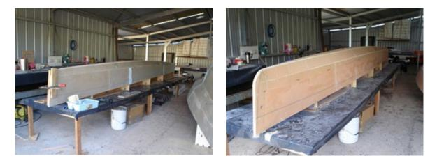
The floats are removed from the frame and taped inside. The floats were levelled and the bulkheads trimmed to fit. All the bulkheads are taped in the floats. A stringer was added in the centre to help the deck hold its shape
