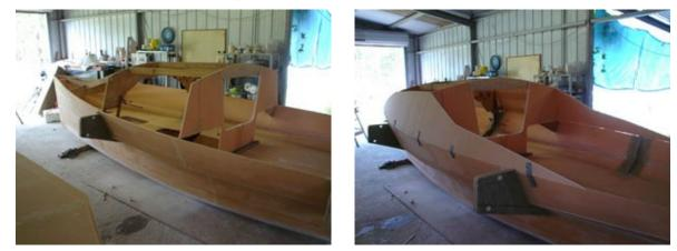
The cabin sides are attached to the frame and the other cabin panels with metal straps. Foam is bent over the frame and attached to temporary pieces of foam attached to the cabin sides. Glass cloth is laid over the foam and wetted out with resin. We use peel ply as well to cut down on finishing later. The edges of the cabin sides and roof are then taped.
