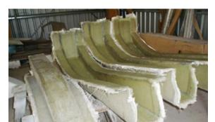
When the beam is removed from the mould it can be trimmed with a diamond disc in an angle grinder.
