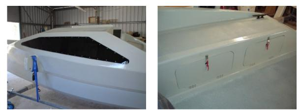
The locker covers are painted, trimmed and attached with hinges. Small pieces of stainless steel are bent and added as latches with some spectra rope added.
