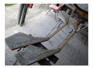
Bulkheads are cut out using the off-sets in the plans. They are made using the same laminate as the panels. They are trimmed if necessary and tacked in place and then filleted and taped in the main hull.
