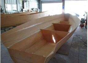
The main beams are taped in. A ring of glass is laminated around the main hull from side to side on the forward and aft beams.
